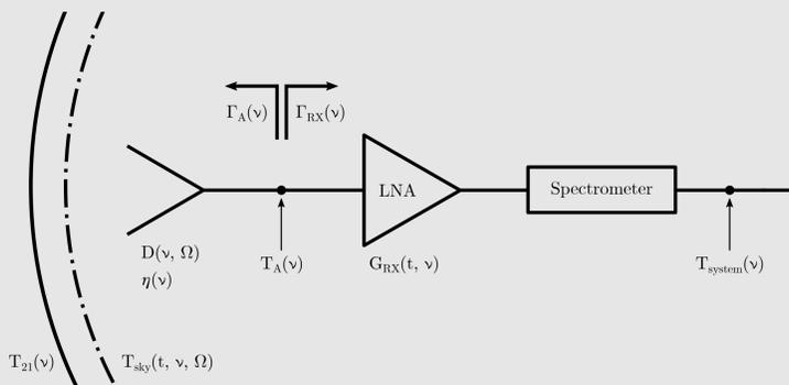
Figure 2. Schematic diagram of the REACH antenna and receiver.
