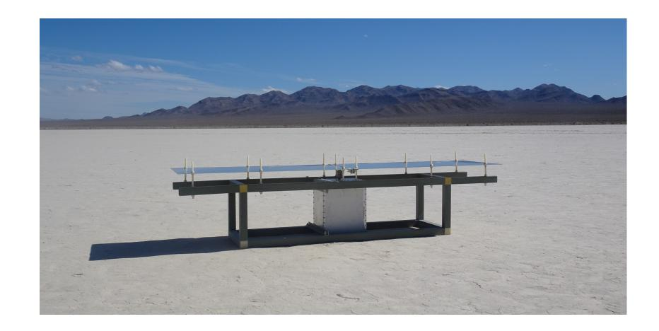
MIST is a portable blade dipole experiment to measure the global signal from cosmic dawn. It does not use a ground plane, which avoids spectral structure induced by reflections from the edge of the ground plane. The tradeoff is the ground underneath the antenna becomes part of the system, and needs to be modelled.
