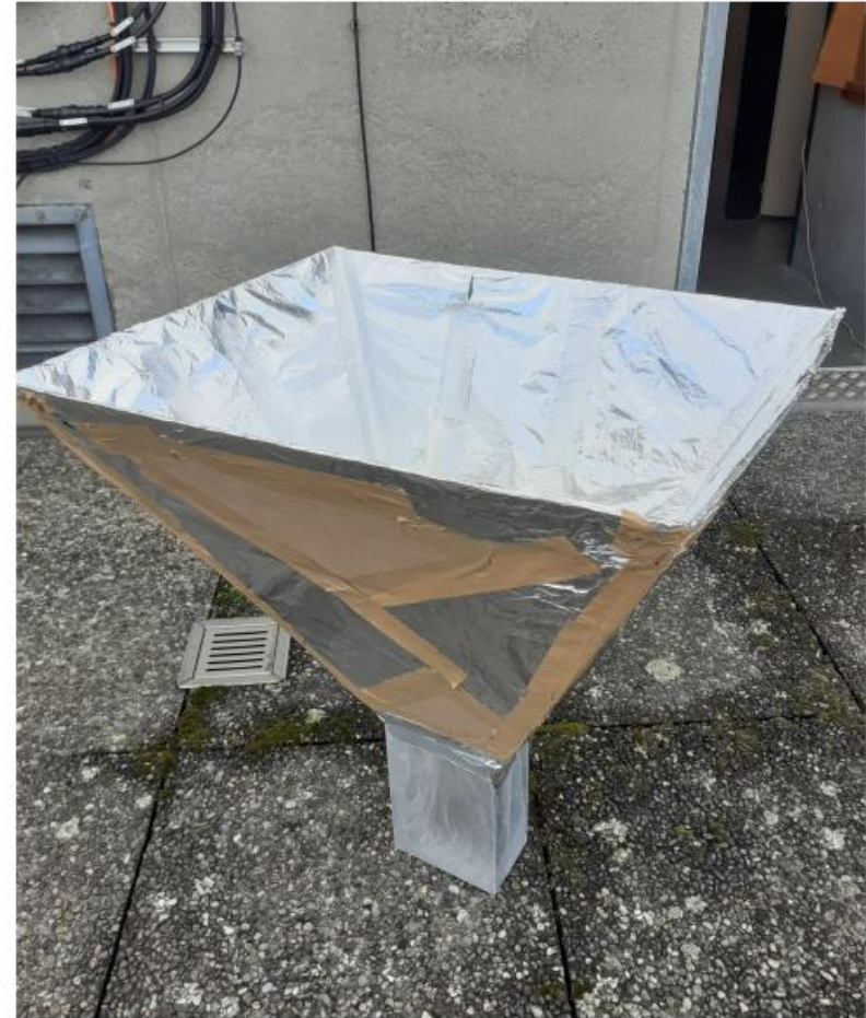
FIG. 7. Photograph of the 2nd attempt at a full radio telescope. This is a rectangular waveguide with a pyramidal horn.
