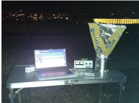
FIG. 6. Photograph of the 1st attempt at a full radio telescope. This was a trial run to see if we could receive signals from various regions in the night sky, such as the Cygnus constellation, which contains Cygnus A, a widely known radio galaxy.
