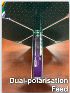
f/0.25 prototype composite dish
