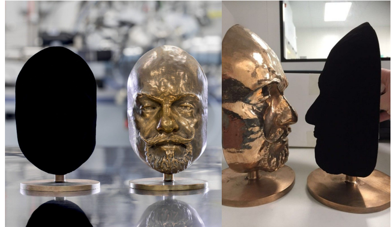
Two identical bronze casts - except one has been coated with Vantablack (Supplied: Surrey NanoSystems)
