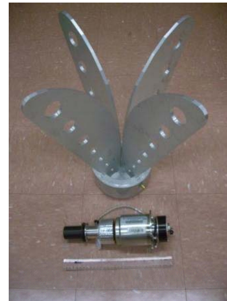
Wide band feed with Stirling cooler (Sandy Weinreb)
