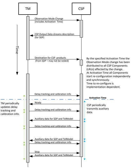
Figure 7-12 Observing Mode Change – Time Sequence Diagram
