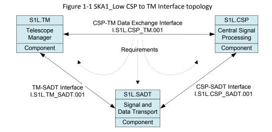
Figure 1-1 shows how interfaces are identified in the SKA1 system.
