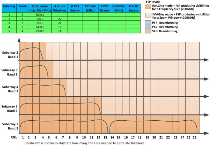
Any frequency slice can be processed on any FSP.
