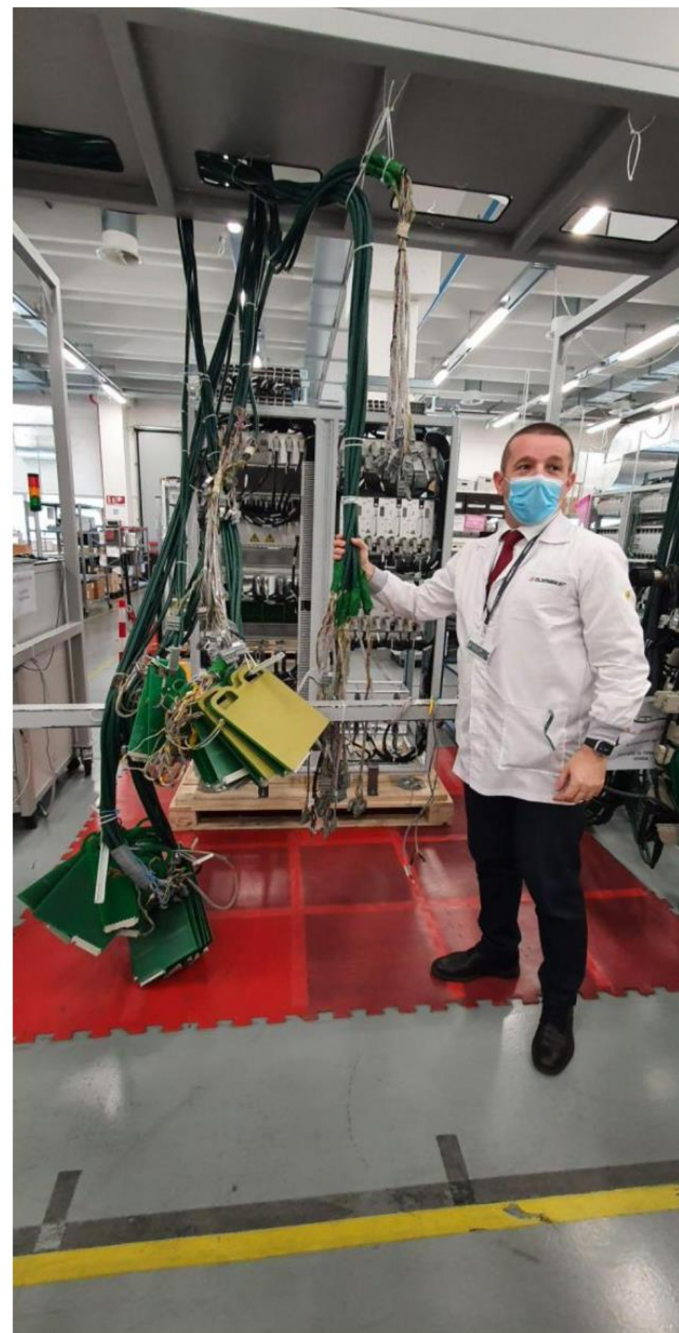
Rack level testing of a railway management system at ELEMASTER
